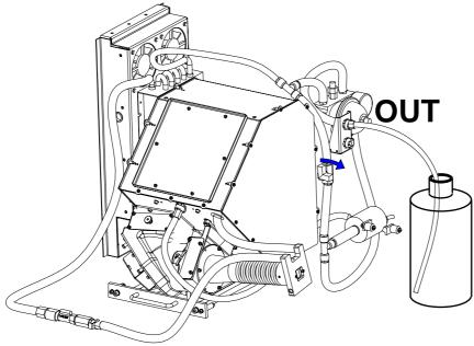
Image 2-6 Drain complete circuit
